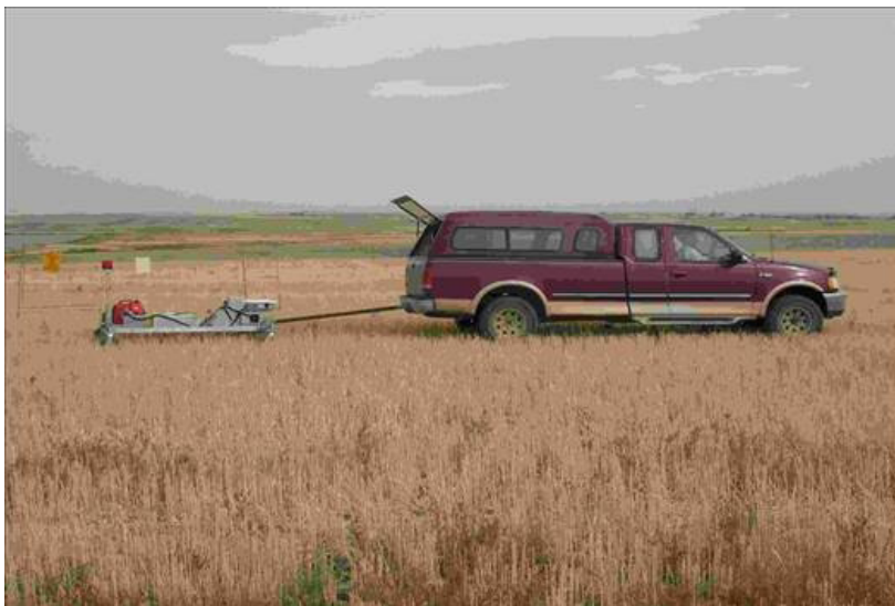
Figure 3. INS system deployed in a wheat field in Montana
