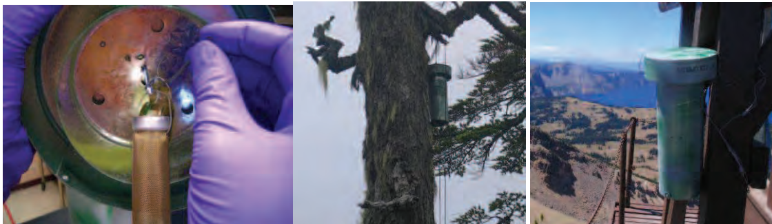
Figure 3-3. Passive Sampler: (a) Hooking resin cartridge to underside of housing cap, (b) Deployment from an exposed tree branch in the Stikine-LeConte Wilderness, and (c) Deployment from a fire tower in Crater Lake National Park.
