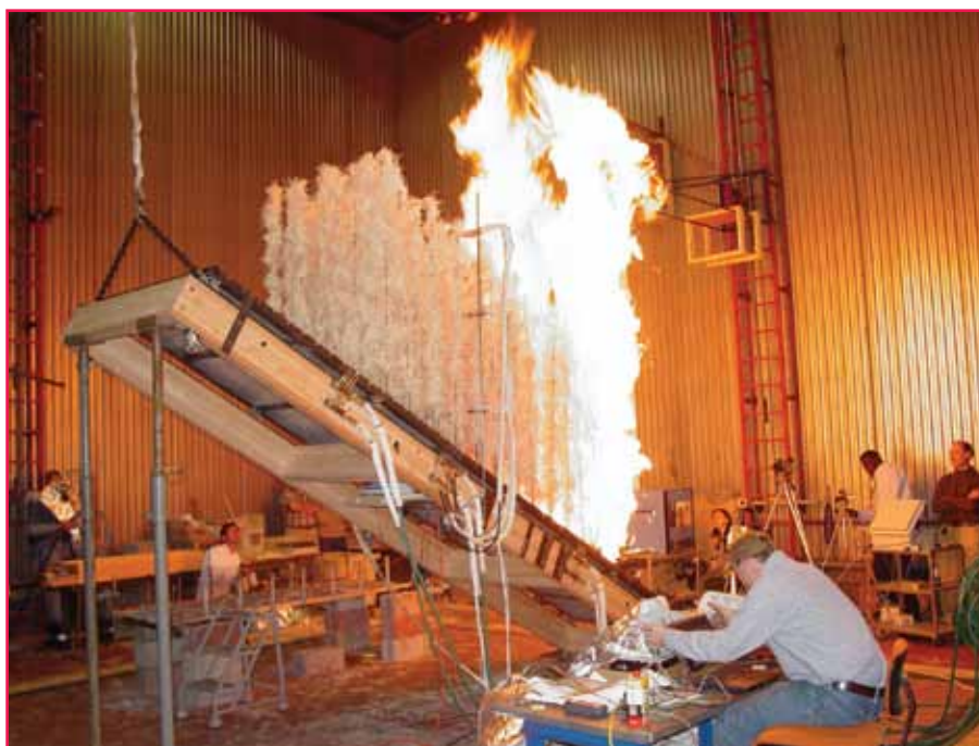
Recent experiments in the fire lab's burn chamber simulate various thresholds and limitations to fire spread on a hillside. Photo: Forest Service.
