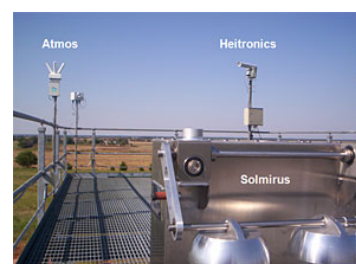
Three of the four instruments deployed in the Infrared Sky Imager Intercomparison Study conducted in 2007 are visible in this photo taken on the Guest Instrument Facility platform at the SGP site. They are the Solmirus All Sky Infrared Visible Analyzer (foreground), Heitronics Nubiscope (top right), and Atmos Cloud Infrared Radiometer-4 (far left).
