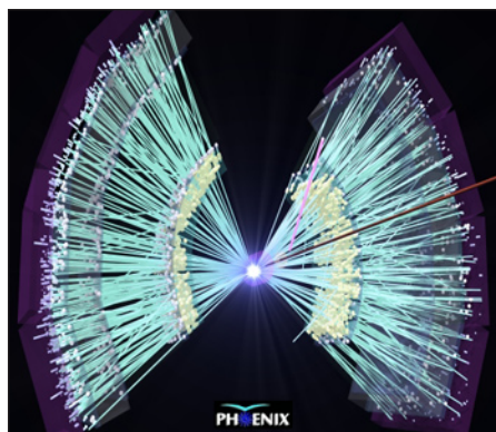
End view of particles emerging from a collision of two beams of gold ions in the PHENIX detector at the Relativistic Heavy Ion Collider at Brookhaven National Laboratory.
