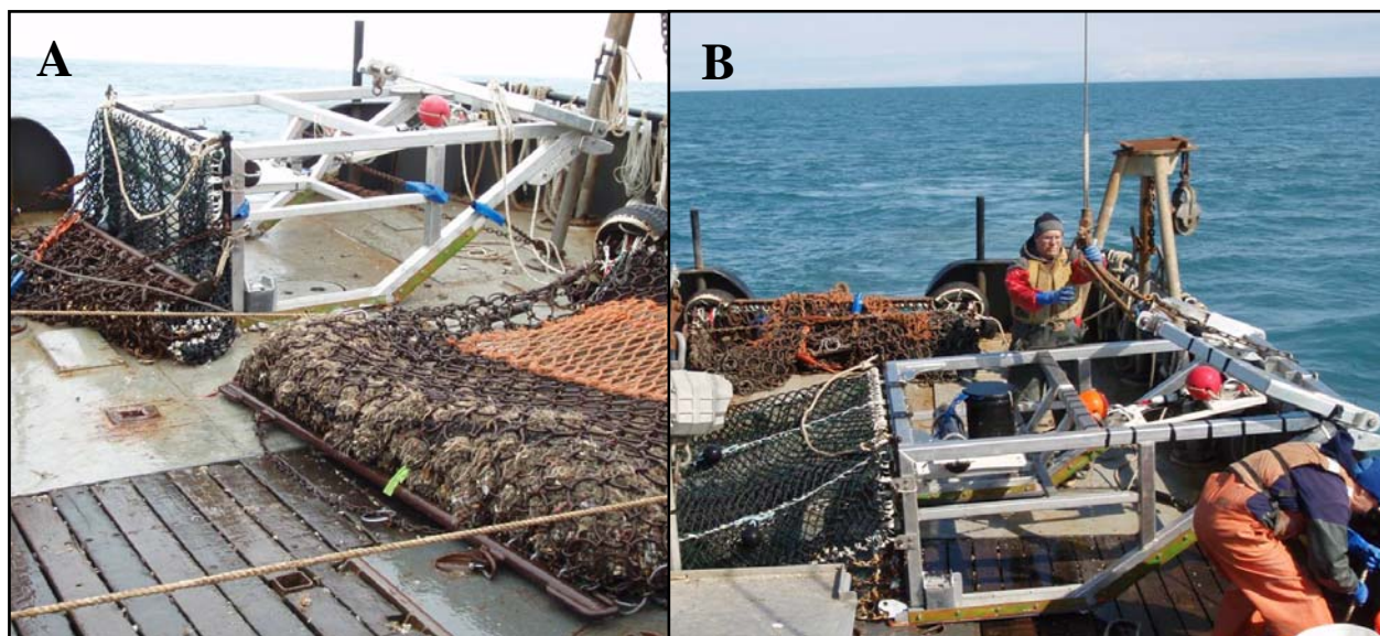
Figure 11 A) Photo of sled-dredge onboard deck of R/V Pandalus, with 8’ dredge bag in foreground; B) ADF&G sled-dredge with bag stretched out on deck after trial tow (8’ dredge can be seen in background).
