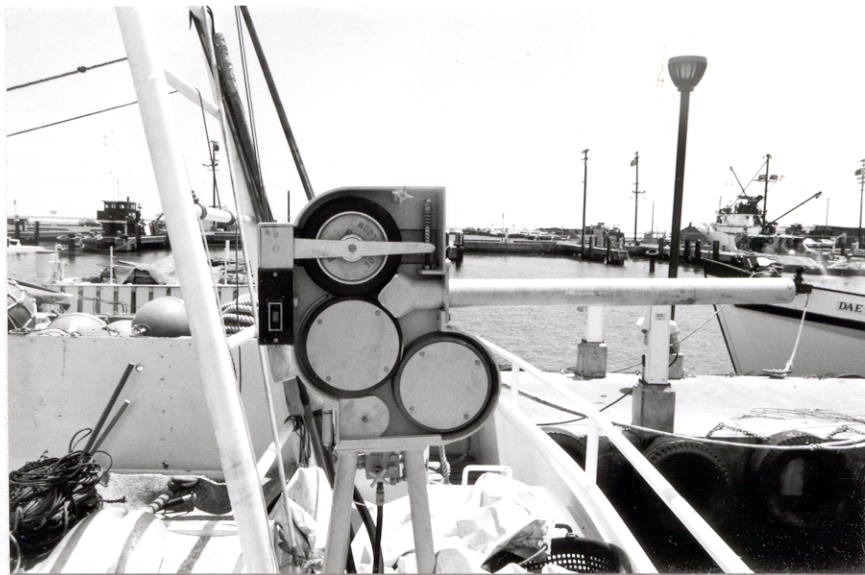
Figure 8.--Monofilament line thrower.
