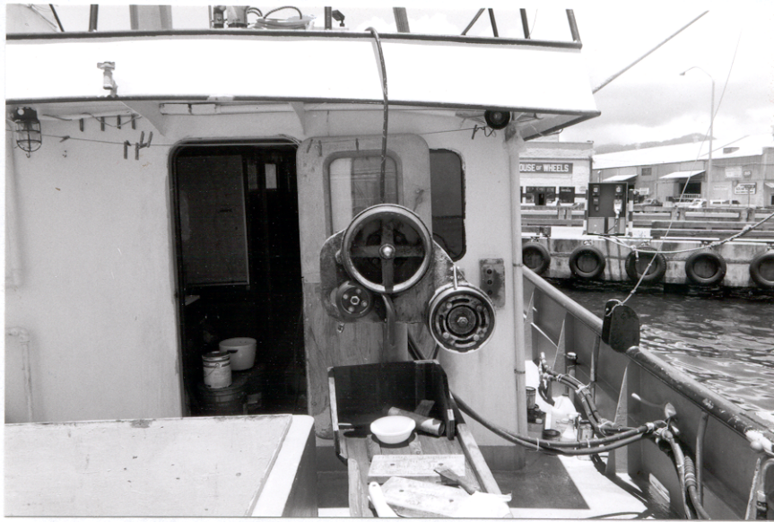
Figure 5.--A mechanical line hauler.
