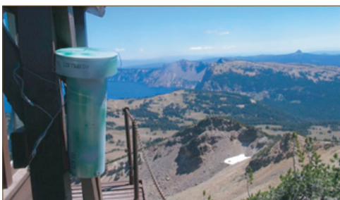
A passive air sampling device (PASD) collects data about airborne contaminants.
