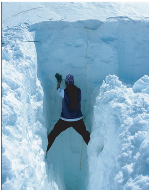
A researcher collects snowpack samples from the sides of the snow pit, avoiding contamination.
