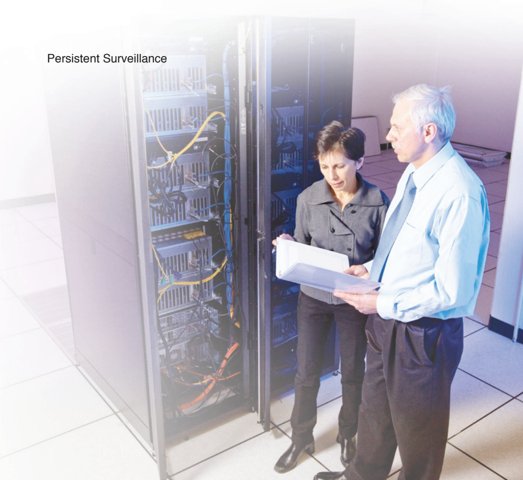
Persistics software is currently housed on a high-density 12-node minicluster, providing an aggregate 40 trillion floating-point operations per second of computing capability. Each node contains a combination of central processing units and seven graphics processing units. Pictured are (left) Sheila Vaidya and Holger Jones.
