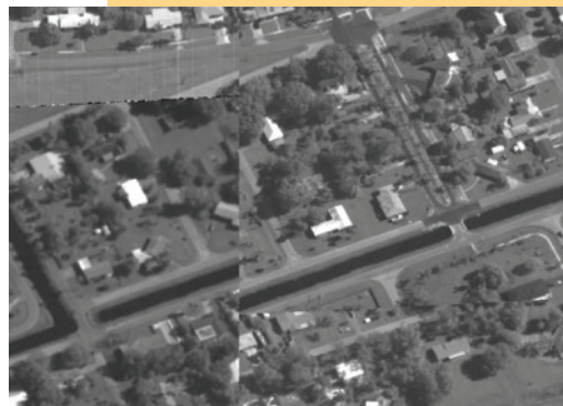
(left) In the manual stitch image, the road does not line up between the collected images. (right) Dense image correspondence corrects for intensity variations between cameras to provide a seamless image.
