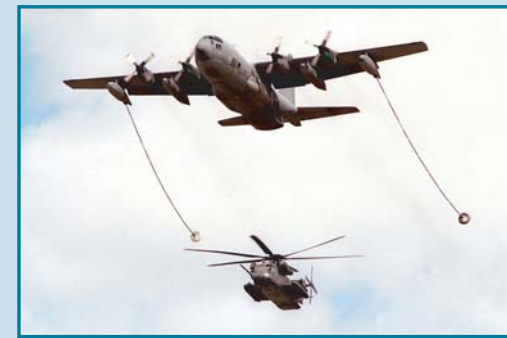
Aerial Refueling - Most MC-130 aircraft have capability to refuel special operations helicopters and CV-22 Osprey.
