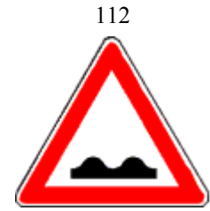
Rough Road. Indicates uneven stretches of road.
