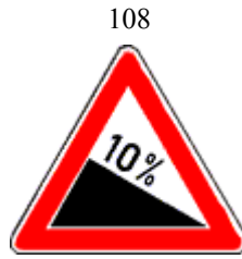
Dangerous Downgrade. Posted before steep downgrades; indicates degree of downgrade.
