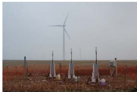
Lidar wind speed/turbulence measurements to heights of ~200 m
