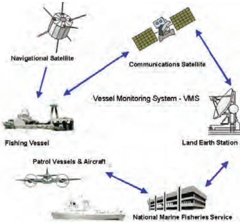
Schematic of how VMS works.
