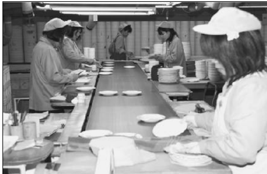
The dishes move along the table, each getting inspected for flaws and cracks, ensuring perfection for customers.
