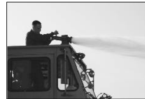
Stallard mans the turret of a P-19A Aircraft Rescue Fire Fighting truck during the daily "wet check." The check ensures that the pumps and hoses are in good working order.
