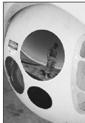
Mounted just under the nose of a Huey helicopter at Al Asad, Iraq, the BRITE Star thermal imaging and laser designation system allows the UH-1N to support a variety of imaging and targeting missions, particularly laser designating for Hellfire missiles.
