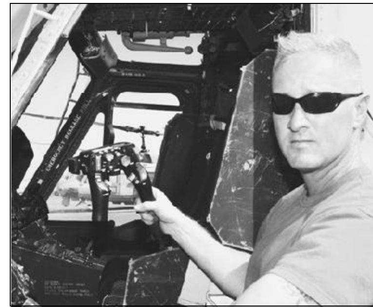
Chief Warrant Officer 2 Michael W. Reed, maintenance officer, Marine Light Attack Helicopter Squadron 169, shows off the remote control for the BRITE Star thermal imaging and laser designation system aboard one of the squadron's UH-1N Huey helicopters at Al Asad, Iraq.
