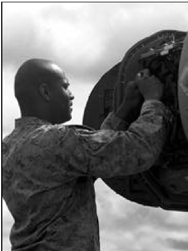
Cpl. Randy Saulsberry, Marine All-Weather Fighter Attack Squadron 225, works to repair an F/A-18D radar. The squadron lent its assets to Northern Edge 2004, May 31.
