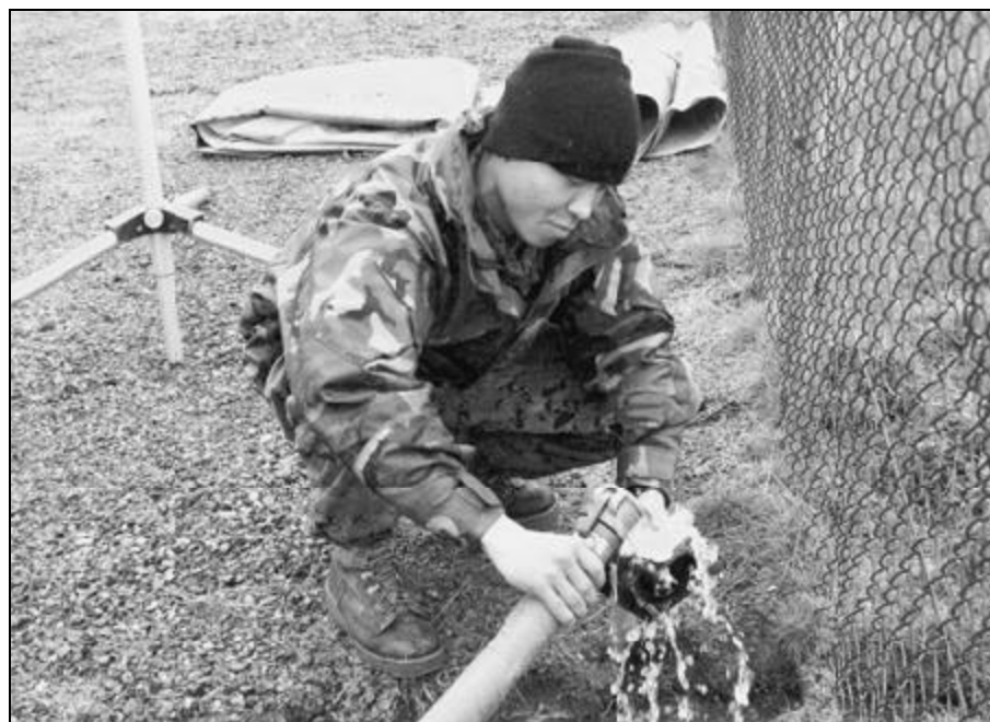
Pfc. Tseten D. Lama uses the total dissolved solids meter to determine the purity of the water.
