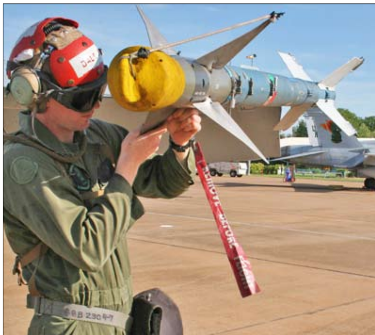
Lance Cpl. Larry S. Minks, a Marine All-Weather Fighter Attack Squadron 121 aviation ordnance technician, adjusts the front fin of an AIM-9M training missile attached to the wing of an F-18 fighter jet. Photo by Lance Cpl. Dan Negrete
