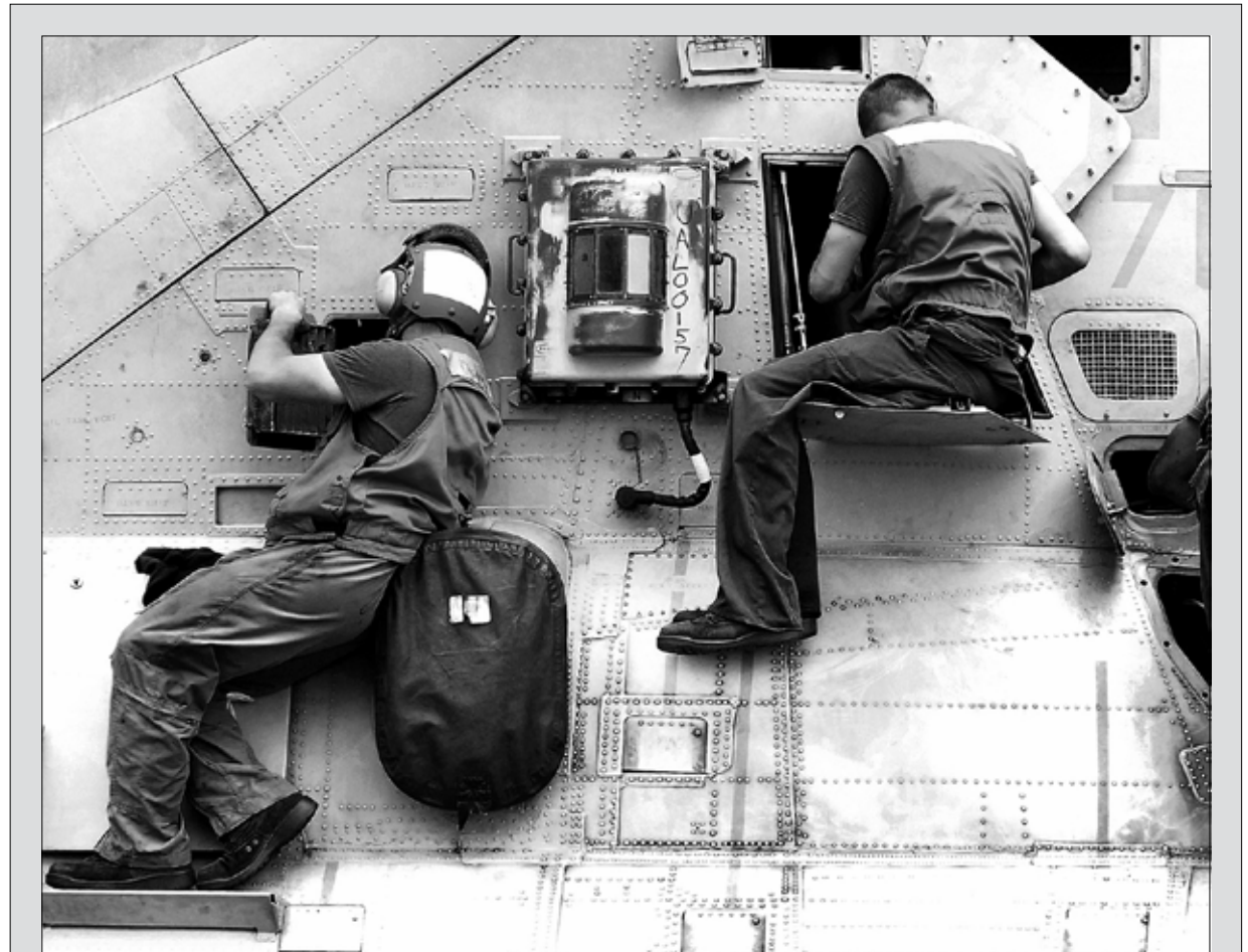
U.S. Marines cling to small ledges on the tail of a Sea Knight helicopter to remove dirt and debris from within the aircraft during an agricultural wash on the flight deck of the amphibious assault ship USS Peleliu in the Gulf of Aden, Sept. 4. Photo by Petty Officer 2nd Class Dustin Kelling
