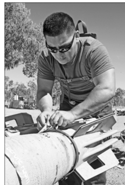
Cpl. Fernando Banda, a MALS-12 ordnance technician, attaches a dexter clip to a BSU-86 fin on a high-explosive 500-pound bomb. The release, if used by the squadron, will allow the fins to open up during free fall and create drag, allowing the aircraft to escape bomb fragmentation. Photo by Lance Cpl. Joseph Marianelli
