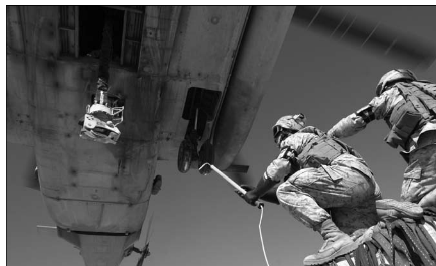
A landing support specialist with Combat Logistics Battalion 6’s Helicopter Support Team connects the static wand to the CH-53E Super Stallion to ground the aircraft before rigging the external load.
