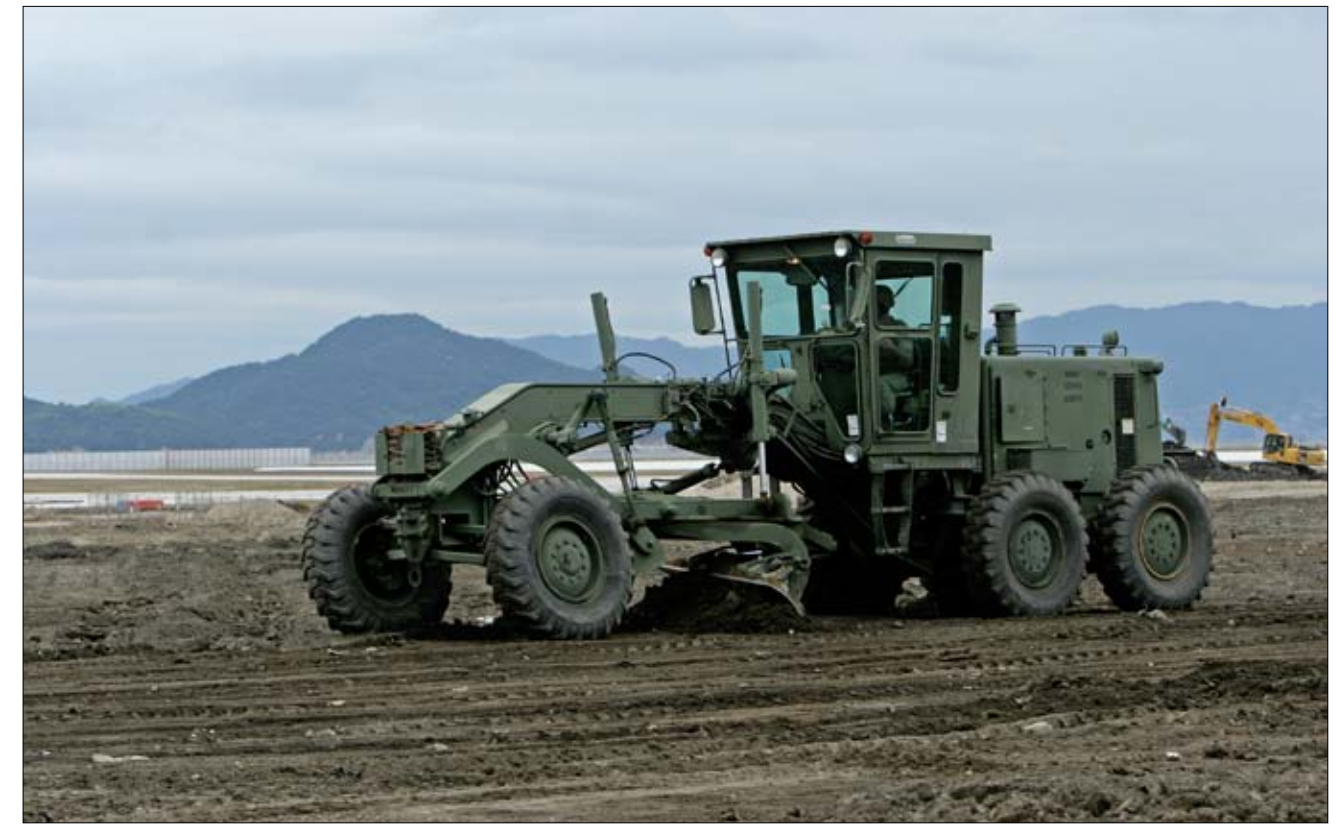
Pfc. Ryan C. Caspary, a Marine Wing Support Squadron 171 heavy equipment operator, operates a grater to level out some ground during a five-week-long exercise Oct. 18 - Nov. 19 at a temporary dig site here. Approximately 15 heavy equipment Marines were able to participate during this rare dig site exercise.
