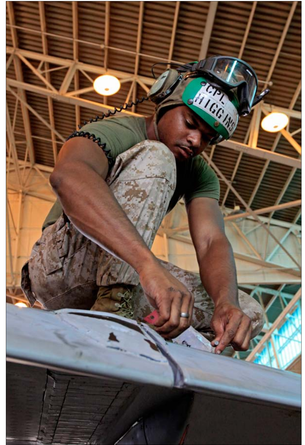
Cpl. William Higgins, fixed-wing airframes aircraft mechanic with Marine All-Weather Fighter Attack Squadron 224, overlooks flight surfaces on an F/A-18 Hornet jet during a phase Bravo inspection here Oct. 5. A Bravo inspection requires multiple electrical and mechanical components to be taken apart, undone and then re-installed. Inspections must be done on an aircraft every time it accumulates 200 flying hours.
