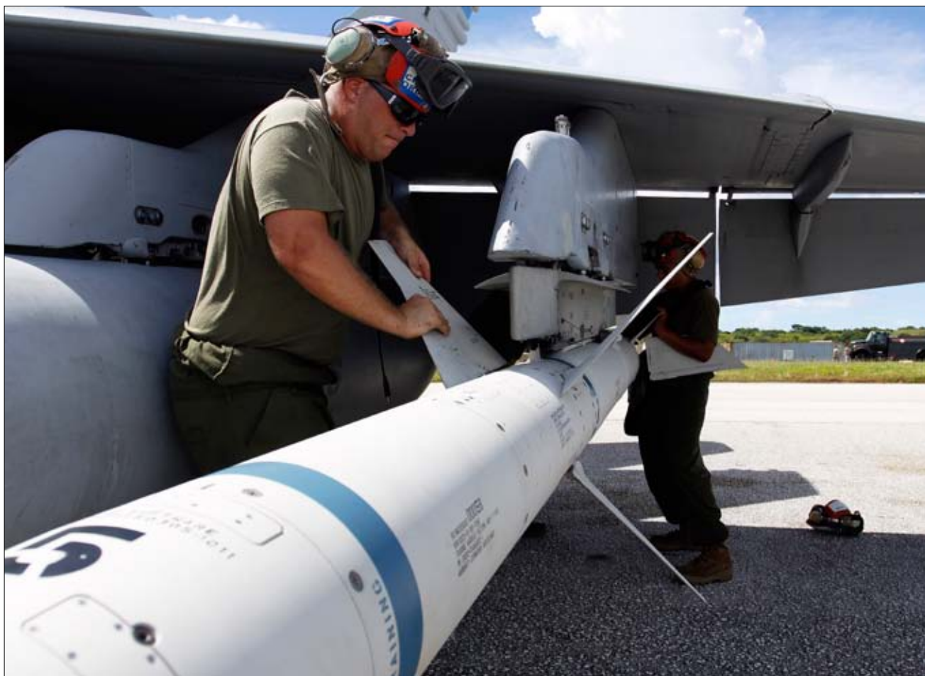
ANDERSEN AIR FORCE BASE, Guam — Cpl. Michael Krenz, a Marine All Weather Fighter Attack Squadron 225 aviation ordnance technician, adjusts the wings of an Air-to-Ground 88 High-speed Anti-Radiation Missile at the flight line here during exercise Valiant Shield 2010, Sept. 16. The F/A-18 to which the AGM-88 HARM is attached to is slated to participate in a Valiant Shield scenario designed to improve joint operation proficiency between all military services involved.
