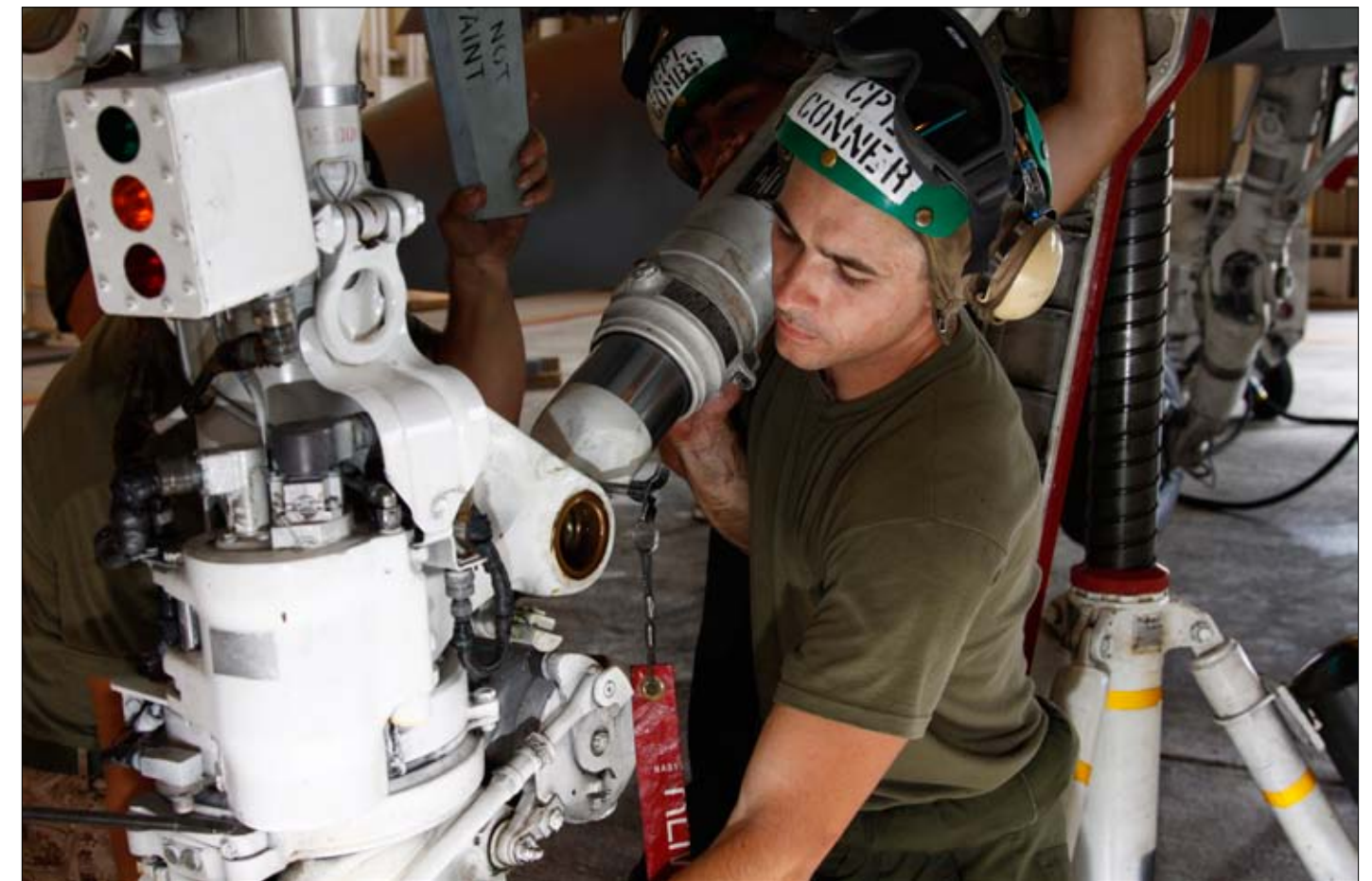
Cpl. Andrew Conner, a Marine All-Weather Fighter Attack Squadron 224 air framer, lifts the drag brace into place just before another Marine places the required parts to install it during a 364-day inspection here Aug. 30. It took a crew of about five Marines to replace the drag brace on one of the fighting Bengals here.
