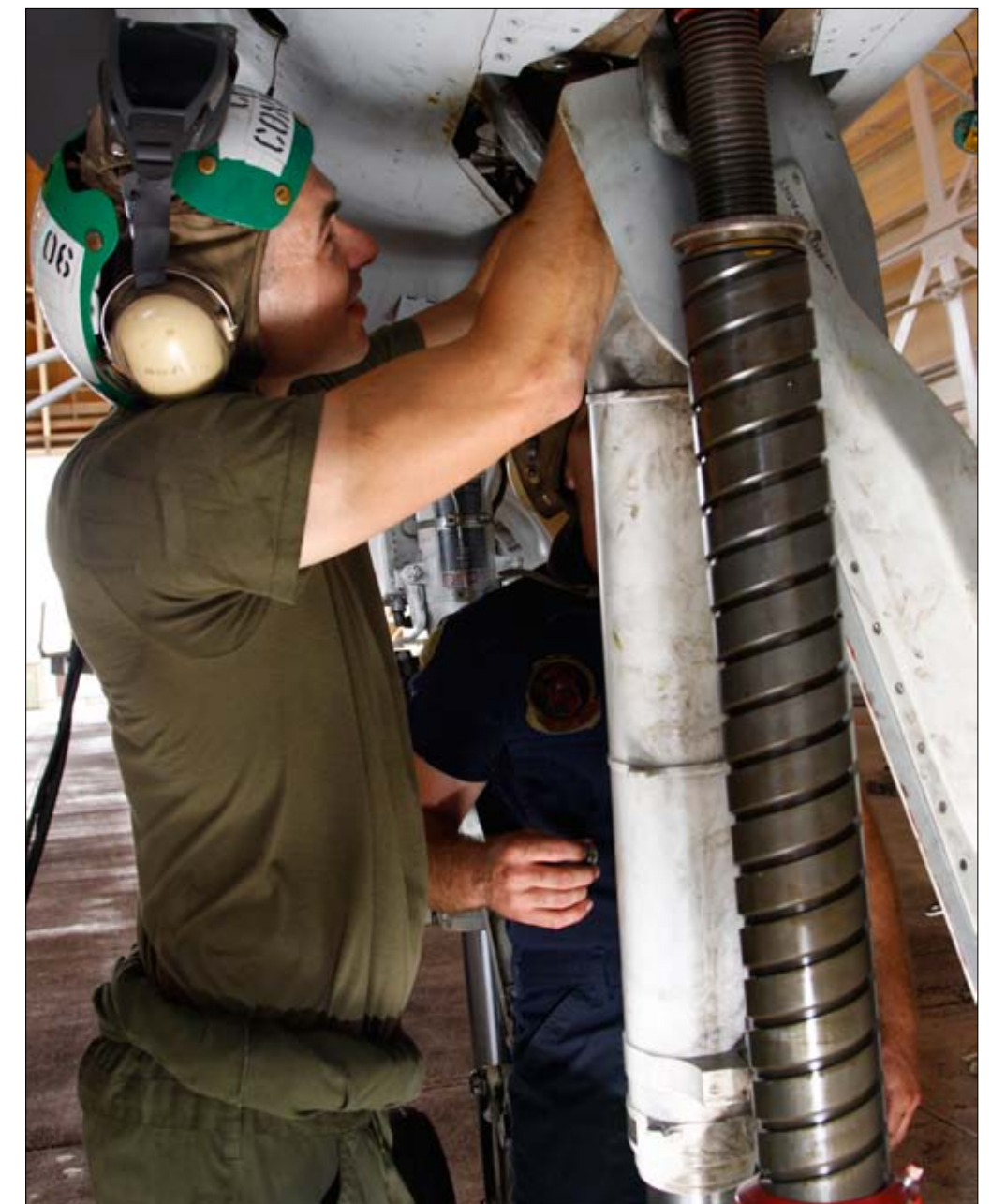
Cpl. Andrew Conner, a Marine All-Weather Fighter Attack Squadron 224 air framer, lifts the drag brace into place just before another Marine places the required parts to install it during a 364-day inspection here Aug. 30. It took a crew of about five Marines to replace the drag brace on one of the fighting Bengals here.
