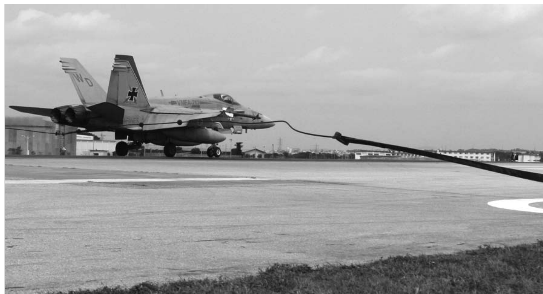
A Marine Fighter Attack Squadron 212 pilot snags the wire with his F/A-18C Hornet during an arrested landing on Marine Corps Air Station Futenma, Okinawa, Feb. 13, 2007. The arrestment gear used at Futenma is the same as what is used on station here.
