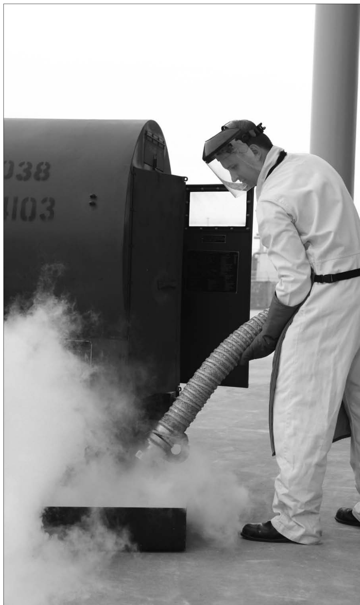
Petty Officer 2nd Class Thomas Armstrong, Station Cryogenics Division technician, purges a cryogenic hose over a liquid oxygen pan at the Navy Cryogenics Division building here July 9. The process of purging clears the hose of excess oxygen or nitrogen particles.
