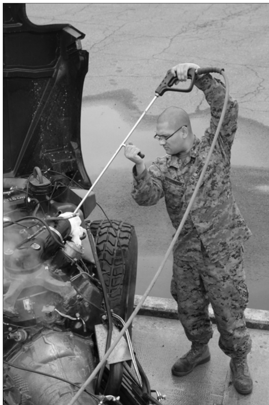
Lance Cpl. Juan Antonio Mayorodriguez, a Combat Logistics Company 36 heavy duty equipment mechanic here, pressure-washes a humvee frame before it is sent for repair. The humvee is separated into pieces so workers can replace the body wiring harness.
