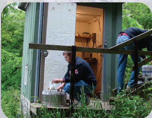
Collecting samples at the Melmore stream gage on Honey Creek. Since 1976, 16,500 samples have been analyzed for nutrient and sediment export at this station. Photo by Ellen Ewing
