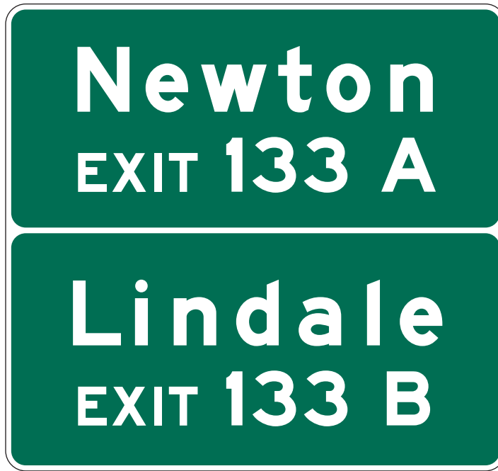
Figure 2E-17. Supplemental Guide Signs for Multi-exit Interchanges
