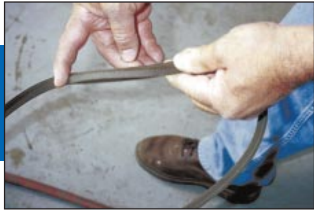
Periodically check your engine belts for cracks — a sign the belt should be replaced soon.
