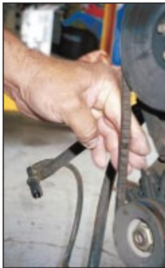
Look for “feathering” or chunks missing from the belt.
