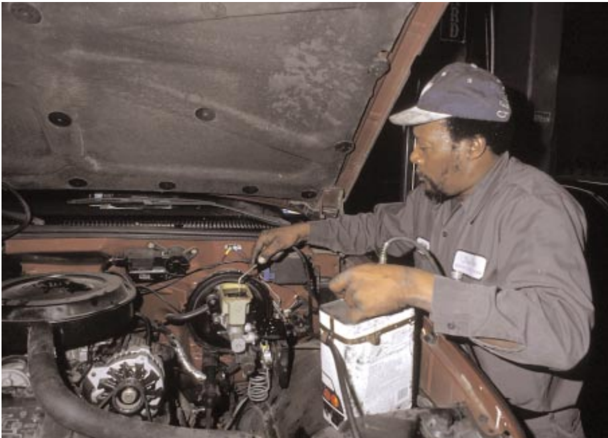
During his under-the-hood checks, the mechanic tops off the brake fluid reservoir.
