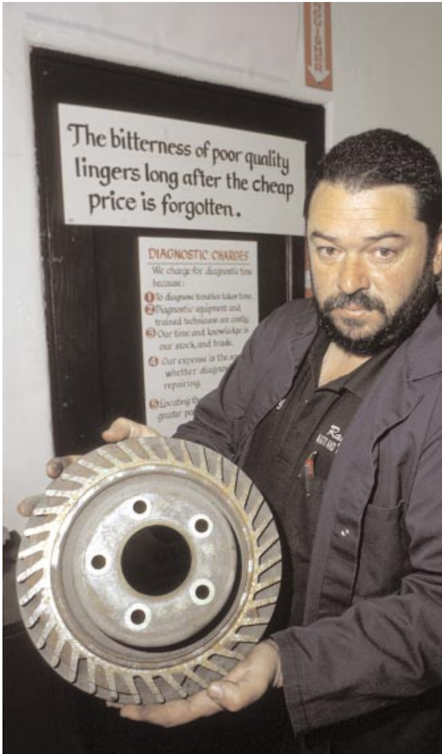
Jerry Haag displays a disc brake rotor from a used car. The rotor is worn all the way through to the cooling fins. Haag has seen used cars offered for sale with disc brakes in the same condition.
