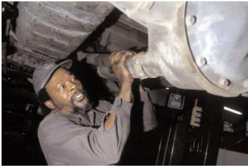
The mechanic checks a vehicle’s drive shaft to ensure the universal joints are not worn out.
