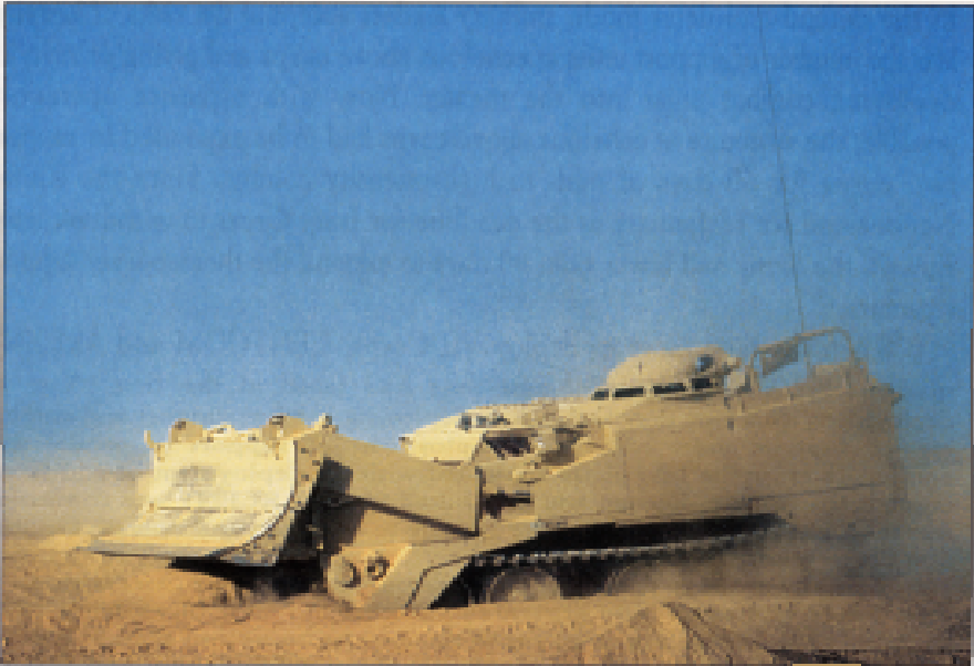
Soldiers of B Company, 5th Engineer Battalion, attached to the 24th Infantry Division use the M-9 armored combat earthmover.
