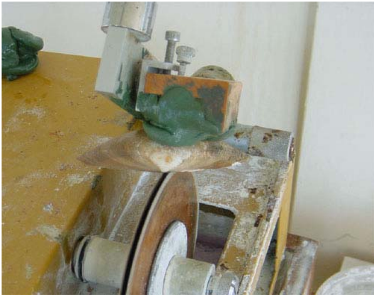
Figure 9. A surfclam shell positioned against two diamond-impregnated blades used to cut chondrophore sections for aging Atlantic surfclam at the NEFSC (photograph provided by J. Burnett, NEFSC).
