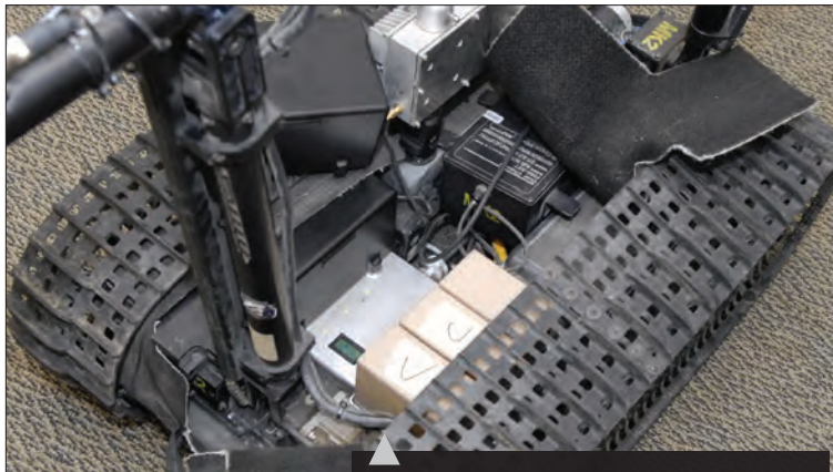
The TBM adapter replaces standard Talon robot battery with six BB2590s.
