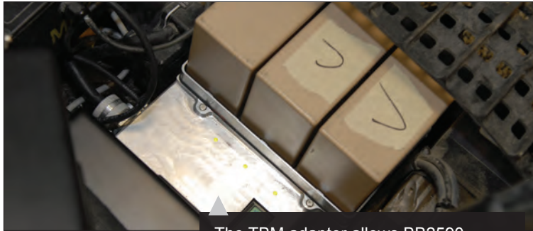
The TBM adapter allows BB2590 batteries to power the Talon EOD robot.
