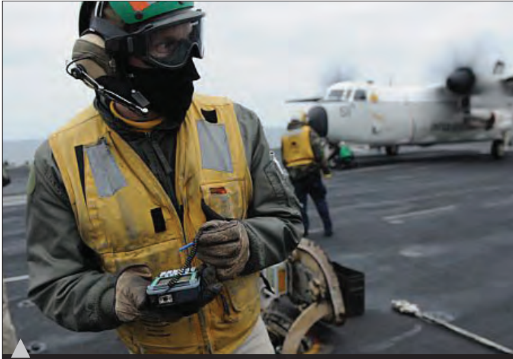
Lt. Andrew Wiese evaluates a catapult capacity selector valve (CSV) calculator provided by the Office of Naval Research during flight operations aboard the aircraft carrier USS Harry S. Truman (CVN 75).
