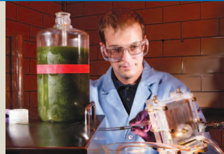
Greg Goddard works on a technique to extract algae's energy-rich lipids and refine them into biofuel, using a new ultrasonic field technology adapted from LANL's award-winning Acoustic Flow Cytometer.
