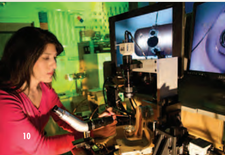
Laida Valdez attaches a shield to a target at LANL's Los Alamos Neutron Science Center (LANSCE). Using a cat whisker, Valdez applies an ultra-violet curing epoxy to attach the shield.
