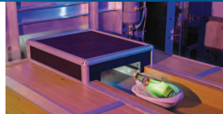
MagViz, a device developed by LANL for airport security use, scans a bottle for dangerous carry-on liquids. LANL won one of its six R&D 100 awards in 2009 for this revolutionary technology.
