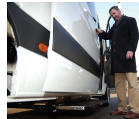
Tim Wood, U.S. Army Garrison Kaiserslautern logistics director, tests the automatic doorstep and movement alarm when a side door opens to one of the 14 vans going to Warrior Transition Units in Europe.
