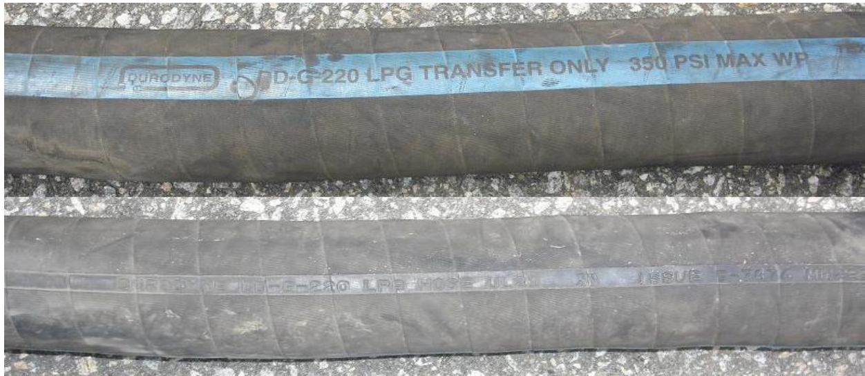
Figure 1: Example of LPG-Use Only Hose Marking
