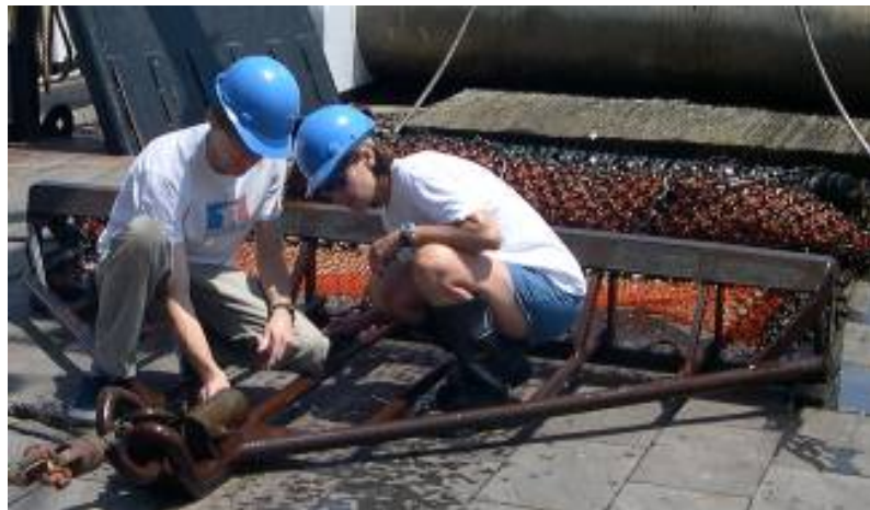
Jakub Kircun teaches Claude Larson how to insert the probe that measures inclination in the top of the dredge equipment.
