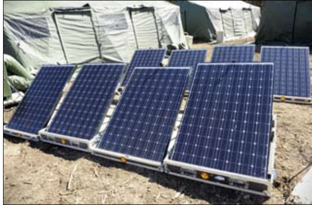
This is illustrative of photovoltaic panels. This particular picture is of a 300-watt photovoltaic battery system, developed by the Office of Naval Research, which can provide continuous power to military in the field. It is designed by the Advanced Power Generation Future Naval Capabilities program located at the Experimental Forward Operating Base at Marine Corps System Command Transportation Demonstration Support Area in Quantico, Va. (U.S. Navy photo by John F. Williams/Released)
