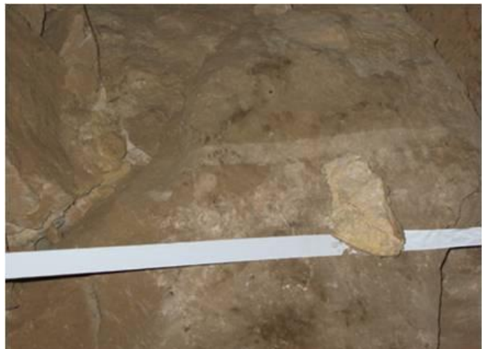
Photo 7. Image taken at a photo-monitoring site showing a light band on the rock where the white flagging tape had previously been. Darker areas on either side of the band are dust accumulation on the limestone (Mike Wiles, JECA).
