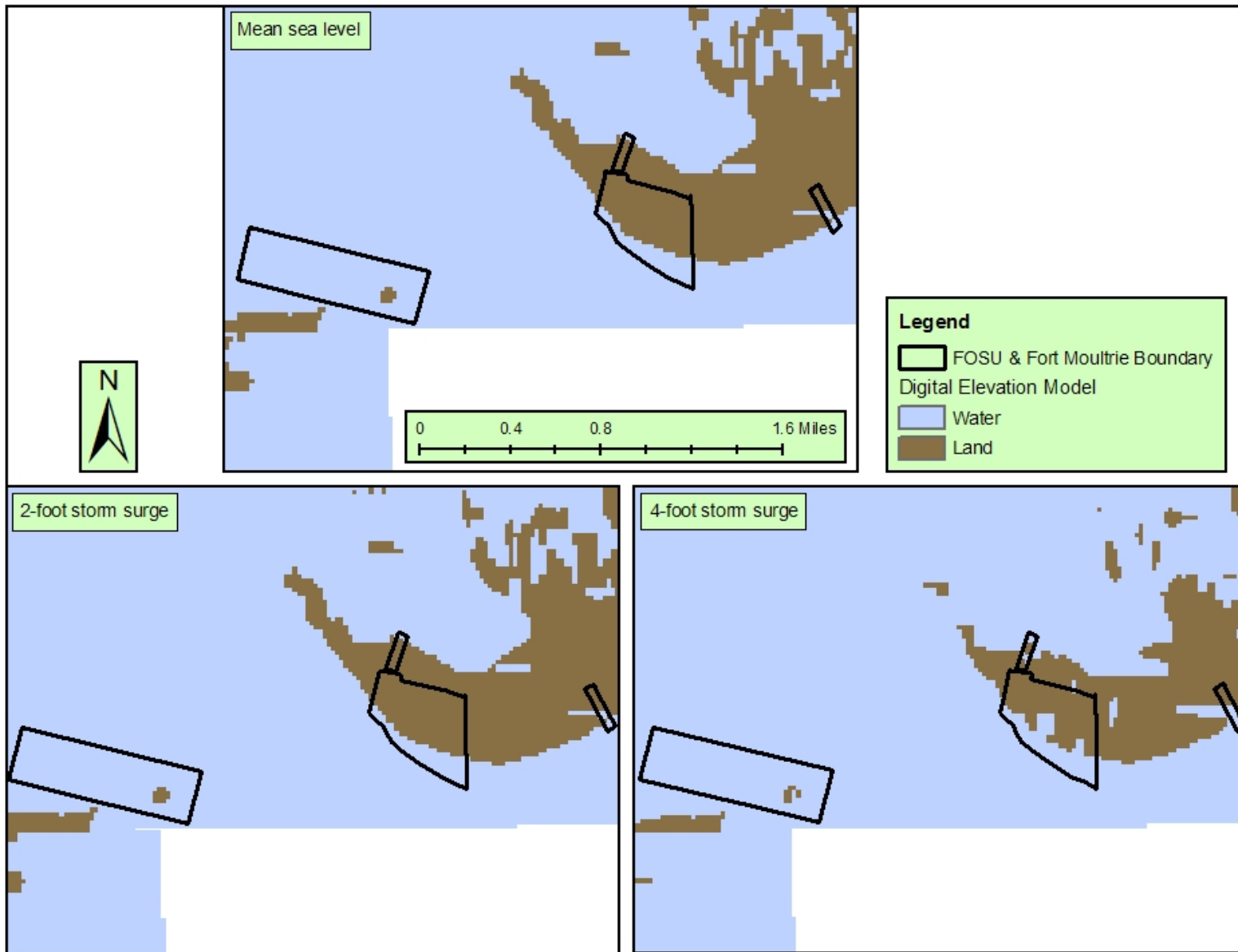
Figure 52. Digital elevation model (DEM) of Fort Sumter NM, Fort Moultrie, and the Coast Guard station showing mean sea level, and approximate two foot, and four foot storm surge.
