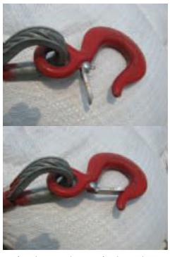
have long been identified as a weak link. We have mitigated this risk by using keeper-less swivels and are phasing keeper-less lead lines into our system. Great awareness report for others. When possible, do not use the lines with keepers. Glad no one was hurt when the net departed the load. Thanks for the discussion item.
