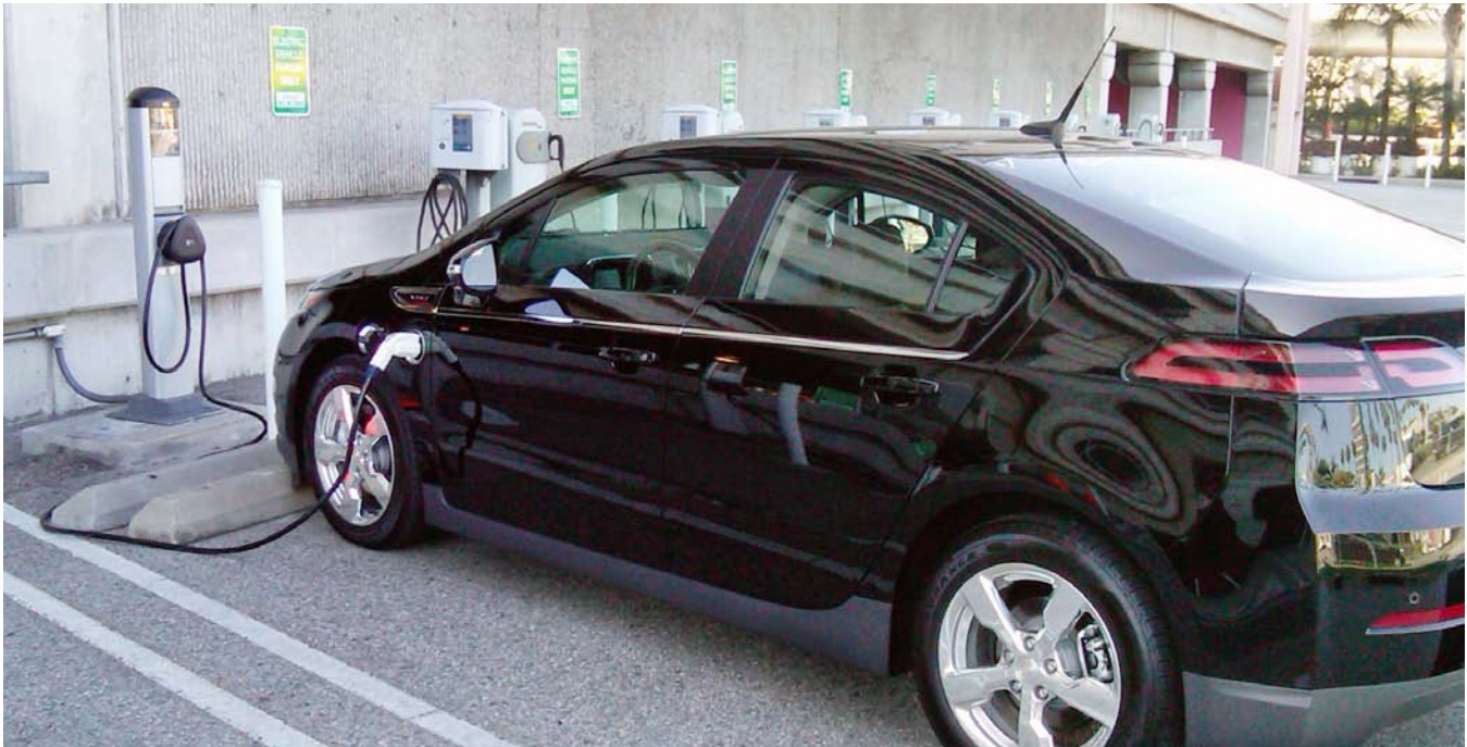
A Chevy Volt charges up with public Level 2 EVSE at Los Angeles International Airport. Photo from Coulomb Technologies
