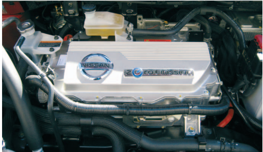
Under the hood of a Nissan Leaf. An EV contains no ICE. Instead, the battery supplies electricity to the electric motor. Photo from Margaret Smith, DOE, NREL/PIX 18215
