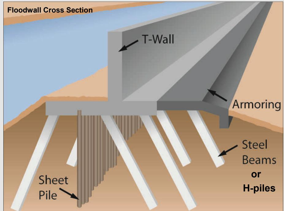
This cross section of a T-wall shows how the floodwall is constructed with steel sheet piles to prevent seepage, and massive H-piles which are placed at an angle to provide strength.
