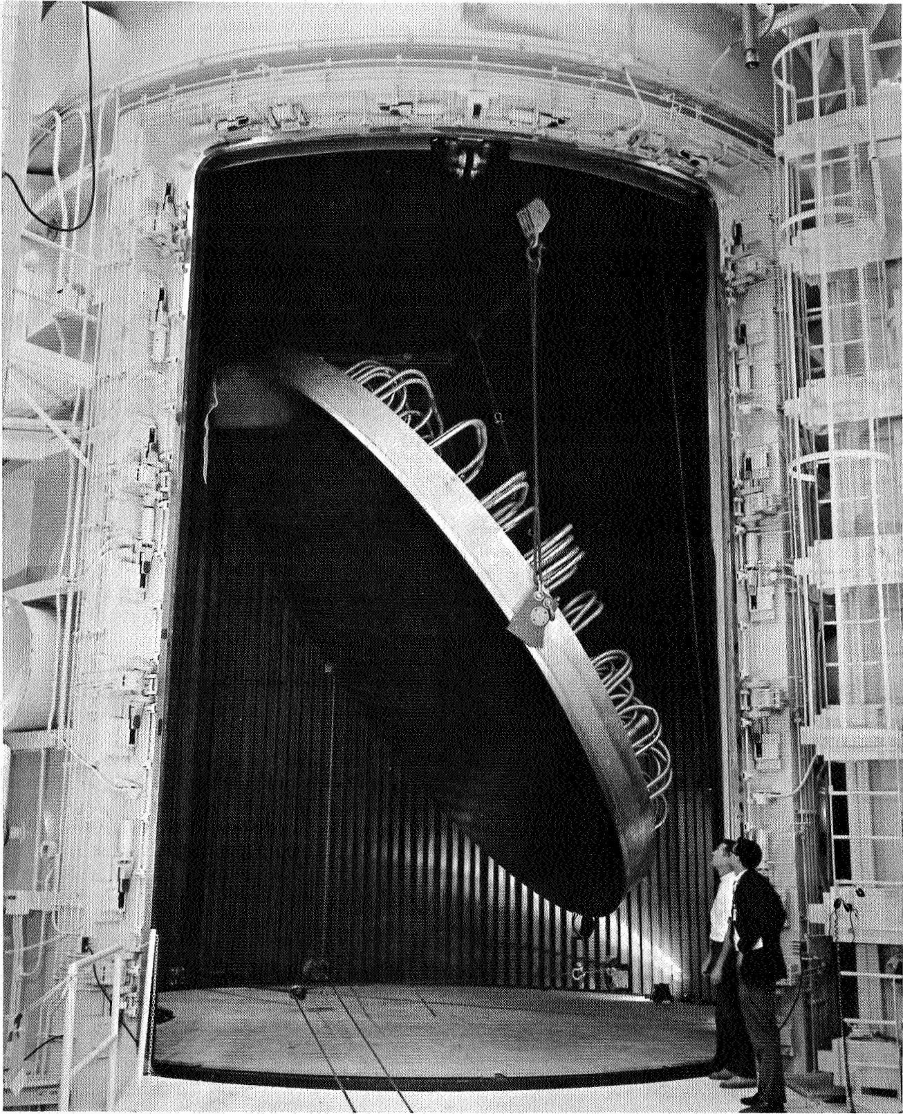
Fig. 4. 23-ft mirror in hoisting position
