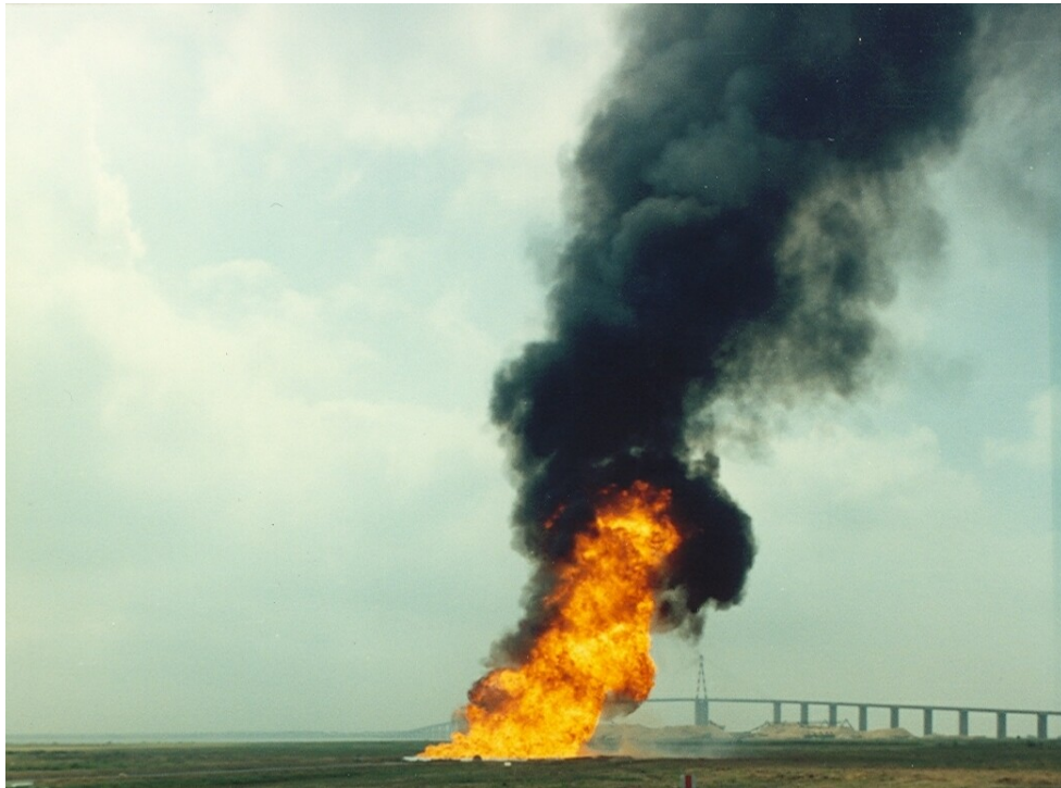
Exhibit 2: 35 m diameter LNG pool on an insulated concrete dike
