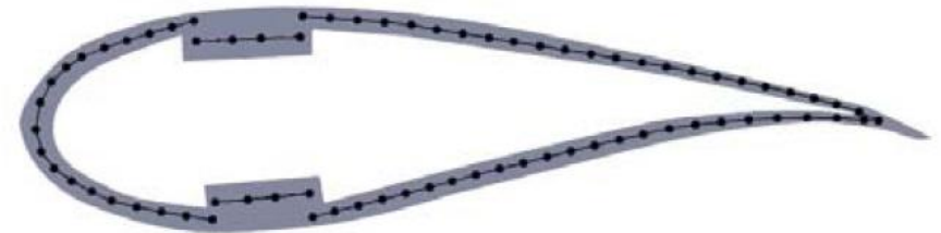
Figure 3. Schematic of physical representation of layered shell elements with nodes offset to the bottom surface. 1
