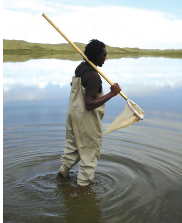
Sampling with a D-net for benthic macroinvertebrates. Photo courtesy of Great Lakes Environmental Center.
