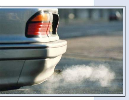
Waste heat claims 60% of the energy generated by an automobile engine.
